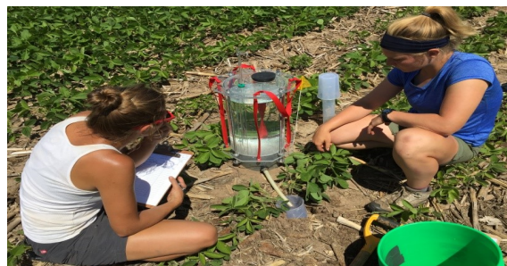
UW-Madison Soil Science graduate students measure the rate of water infiltration to access the effectiveness of gypsum application for reducing soil surface water run-off. (Plymouth)
