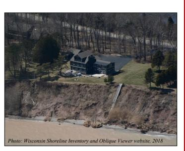
shore. When higher water levels predominate, the water depth closer to shore becomes deeper. As a result, the wave impact increases along the bluff toe, creating more erosion. Although such erosion can be mitigated by properly placed shore protection, it cannot be completely stopped.
